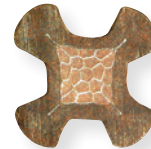
Indenter Crimp Cross-Section Across Axis
